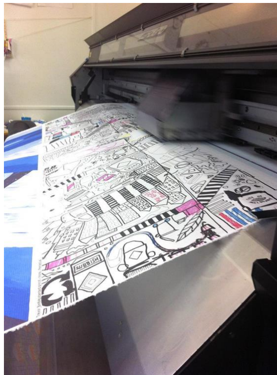
Figure 6.15 Engineered artwork being digitally printed onto 100% cotton fabric for the Helping Hand Bag at Frankie and Swiss, 2015
