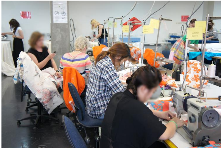
Figure 6.9 RMIT University BA (Textile Design) student production team assembling the tea towels and aprons in the RMIT University fashion workshop. The apron straps were made from cotton tape. The aprons and tea towels were sewn using polyester/cotton thread, photograph by Amanda Magnano, 2012
